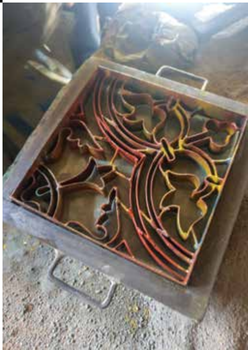
Metal frames used to lay the tiles.
